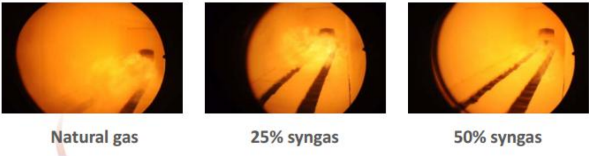
Figure 5 - Combustion visualization through CRIGEN furnace hub [3]
